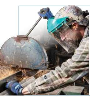
A chop saw is a light, low-horsepower portable machine. Although very similar to a compound miter saw, it is designed for cutting denser materials, like metal bar, tubing or pipe. Chop saw cut-off wheels are designed specifically for this machine with finer grit, softer grades, and reinforcement layers that match the application.
