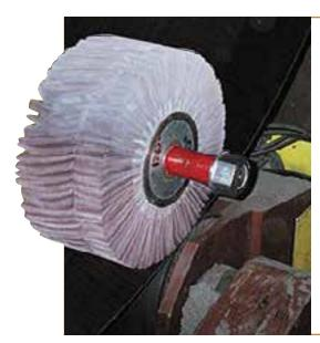
FlexDrum abrasive segments sweep away flaws. Their extreme longevity and perfect balance make them well-suited for automatic as well as offhand use. Hubs and abrasive segments can be combined to fit your job perfectly.
