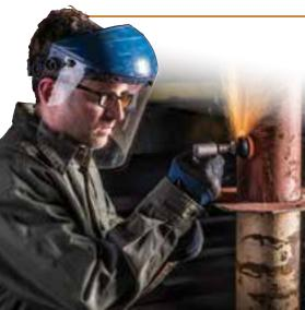
Mini-flap discs are ideal for use in tight spaces. They feature layered flaps which wear away evenly during use exposing new abrasive grain. The lightweight plastic backing helps to absorb vibration. They can help eliminate the conventional 2-step process in grinding edges and removing welds and rust.
