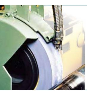
Cylindrical wheels are used most often when the part is held between centers and in chucks. There are three methods of cylindrical grinding: plunge, traverse, and angular.
