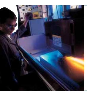
Large surface grinding wheels are generally used to grind flat stock or flat surfaces within a workpiece. These wheels are typically used on horizontal spindle machines. Applications can vary from heavy, rapid stock removal to precision tolerance operations.
