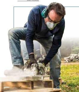
A circular saw uses an abrasive wheel to cut different materials using a rotary motion spinning around an arbor. Norton Circular Saw abrasive cut-off wheels are ideal for use in deburring, cleaning, slotting and cutting all types of metal and masonry.
